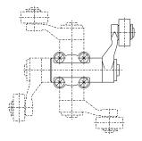
The actuating head can be repositioned by  $4 \times 90^{\circ}$ . Unscrew the four screws of the actuating head (Philips tip profile), reposition the actuating head in the desired position and retighten the four screws (tightening torque 1.5 Nm).
